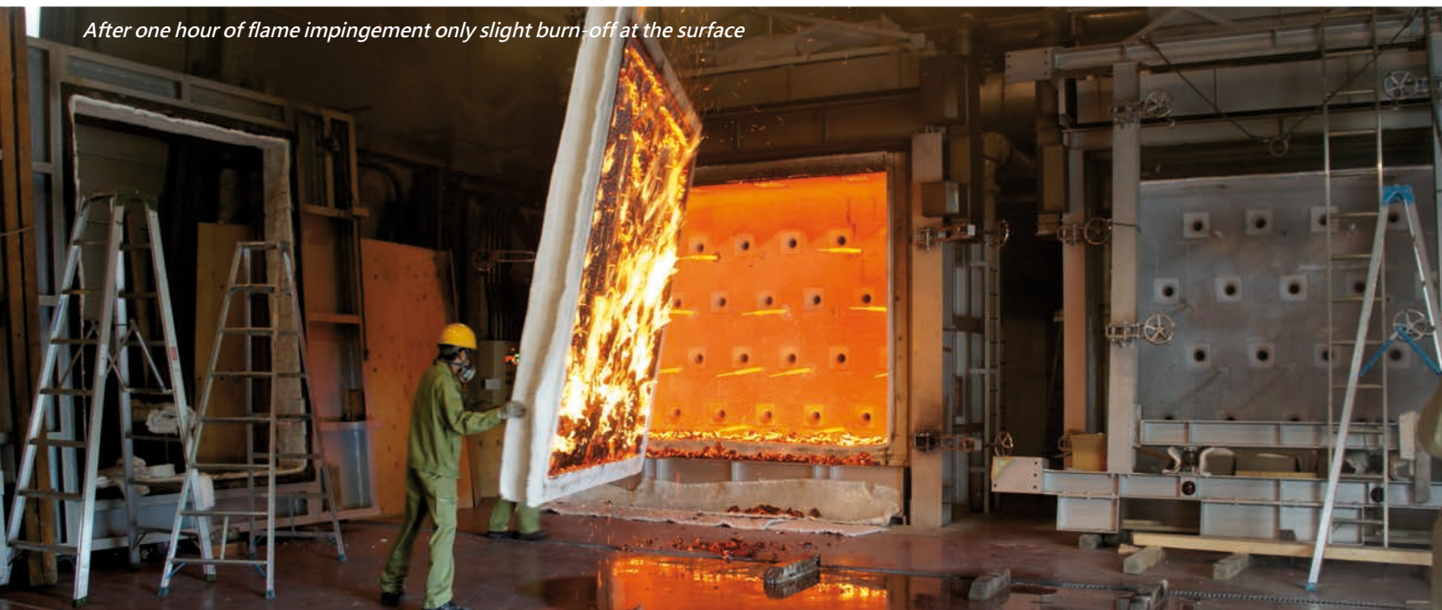
After flame impingement and before extinguishment only minor fire activity
