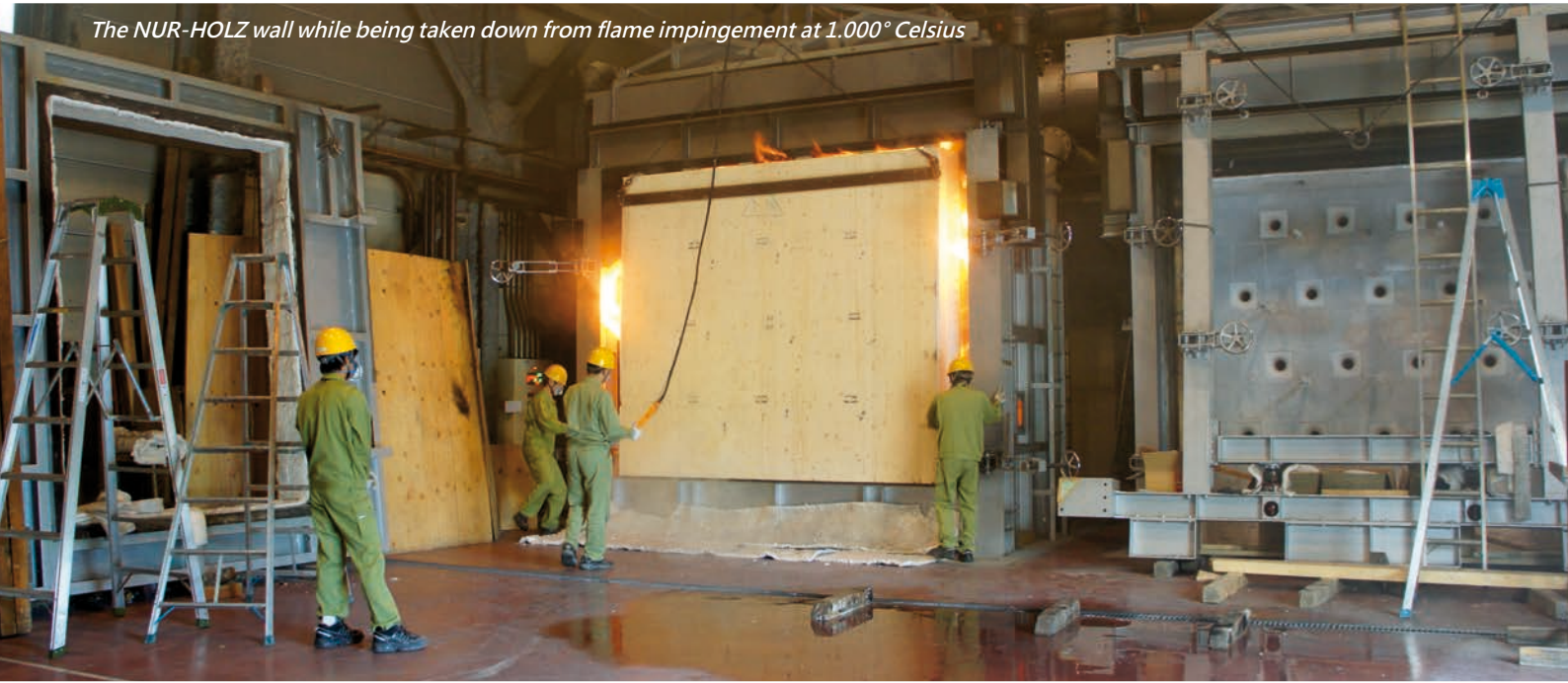
After one hour of flame impingement only slight burn-off at the surface
